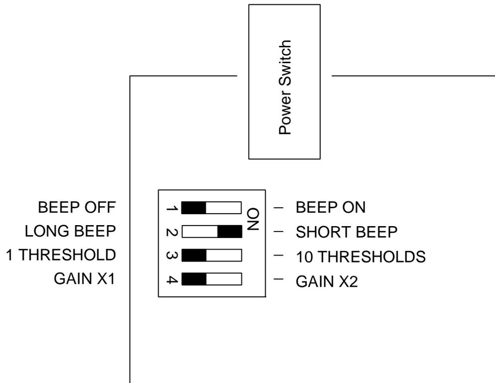
**Figure 4 Internal Programming Switches Normal Settings**
