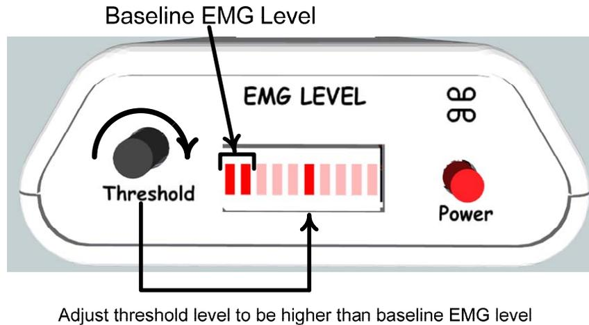
**Figure 2 Threshold Adjustment and Typical Baseline Displays**
